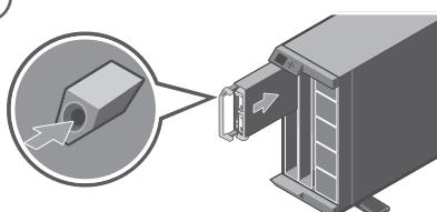
Beginning from the top, install the server module(s) into the enclosure, from left to right.
